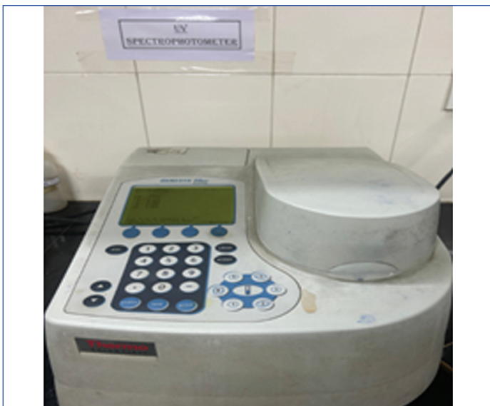
[Table/Fig-10]: UV Spectrophotometer. (Thermo Fisher Scientific GENESYS 10S uv)
